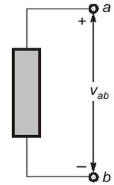
**Fig. :** Polarity of Voltage  $V_{ab}$
