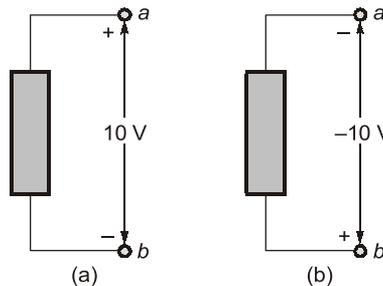
**Fig. :** Two equivalent representations of the same voltage  $V_{ab}$ :
